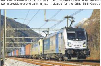
On 1 December 2016 BLS's TRAXX 187 008, on hire from Railpool, leaves the southern portal of the GBT. This class received a new operating permit from BAV for the GBT line on 28 November 2016, following the upgrading of their onboard EBI Cab 2000 ETCS. Those 187s which have not yet been subjected to the upgrade can still use the tunnel, but not in the position of leading locomotives.
