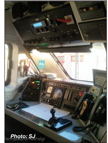
As part of the interior refurbishment new driving consoles are installed in the power car and driving trailer. The edge of the driving console is now curved, thus being more ergonomic (compare with the photo on the right, showing the original console). The new consoles are also prepared for the future installation of on-board ETCS displays. To comply with safety requirements the driver's seat is designed to be pushed back so that the occupant can leave it quickly in an emergency.
