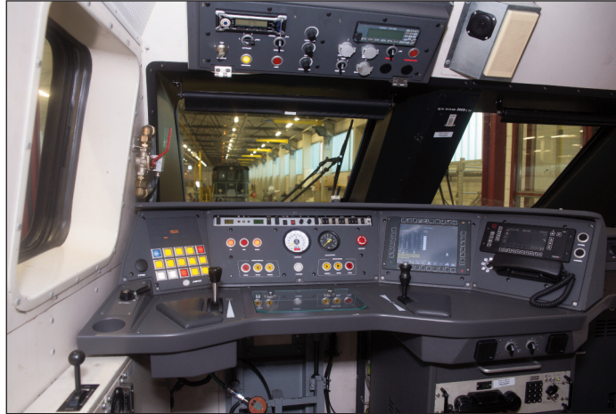
As part of the interior refurbishment new driving consoles are installed in the power car and driving trailer. The edge of the driving console is now curved, thus being more ergonomic (compare with the photo on the right, showing the original console). The new consoles are also prepared for the future installation of on-board ETCS displays. To comply with safety requirements the driver's seat is designed to be pushed back so that the occupant can leave it quickly in an emergency.
