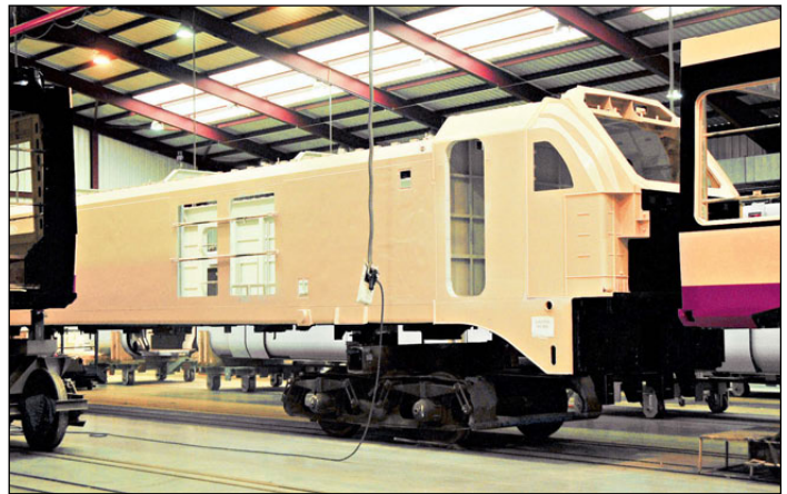
The bodyshell of HVLE's second EURODUAL recently emerged from the paint shop, having received a coating of primer.
