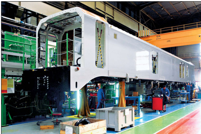
HVLE's first EURODUAL at the final assembly stage.
