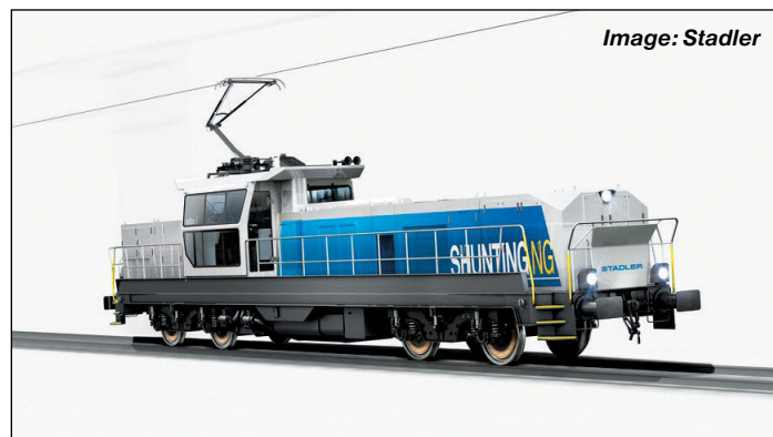
A view of the Stadler's New Generation (NG) shunting locomotive. It is available in three versions: diesel-electric, dual-mode or electro-diesel, and hybrid (diesel/battery).
